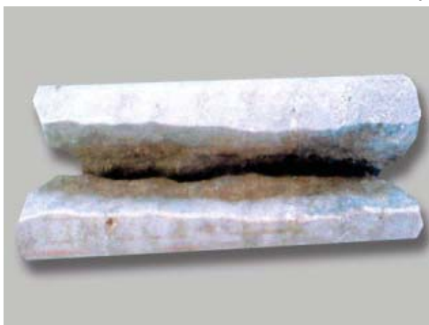
*Core from the BA-15 well shows a typical longitudinal open fracture.
